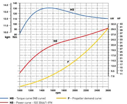
Power ratings refer to engines equipped with air filter, standard muffler, after running-in period at ambient conditions of +25°C, relative humidity 30% and 1 bar. Power levels drop by 1% every 100 m altitude and by 2%
